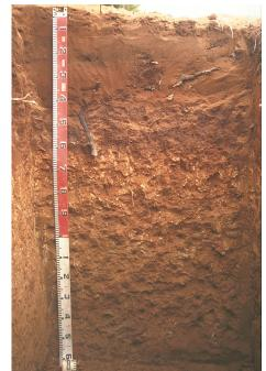
$\textbf{Classification:} \quad \text{Supracalcic, Mesonatric, Red Sodosol; thick, non-gravelly, sandy / clayey, moderate} \\$
