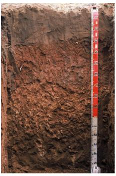
mottled slightly calcareous massive firm medium clay with 2-10% hard carbonate fragments.
